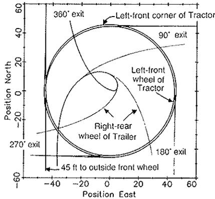
FIGURE 11 Offtracking for a 60-ft tractor-semitrailer vehicle in a 41-ft-radius turn (45 ft to the outside front wheel).
