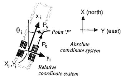
FIGURE 6 Coordinates of arbitrary point P in vehicle unit.
