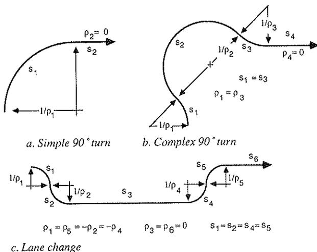
FIGURE 7 Three maneuvers represented as sequences of circular arcs.
