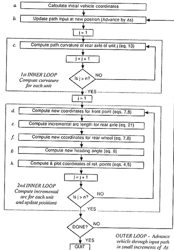
FIGURE 5 Flow chart for offtracking computation method.
