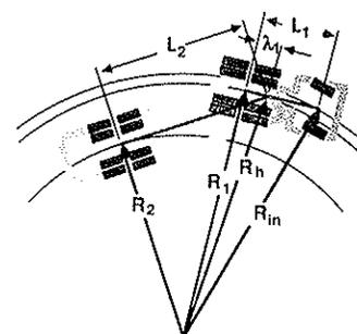
FIGURE 4 Use of the Pythagorean theorem to analyze maximum (steady-state) offtracking of a tractor-semitrailer in a constant-radius turn.
