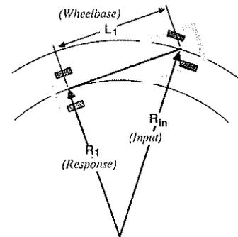
FIGURE 3 Use of the Pythagorean theorem to compute maximum (steady-state) offtracking in a constant-radius turn.
