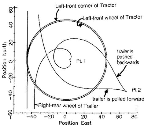
FIGURE 13 Example of a trailer backing up when attempting a continued short-radius turn.
