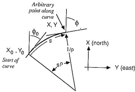
FIGURE 8 Coordinates along a constant-radius curve.
